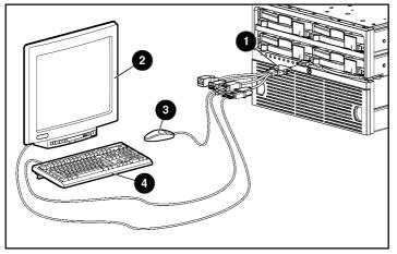
Figure 2-5: Directly accessing a configured server blade
